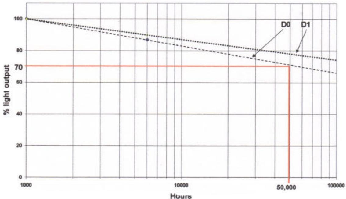
*Lumen Maintenance For CR40RGB Per LRC LED Life Test Vol1 (ENG1210 and 1221)*
